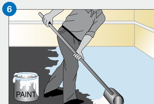
Finish with 2 coats of suitable paint.
